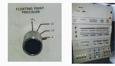
Ken Shirriff: Want to adjust your computer's floating point precision by turning a knob? You could do that on the System/360 Model 44
