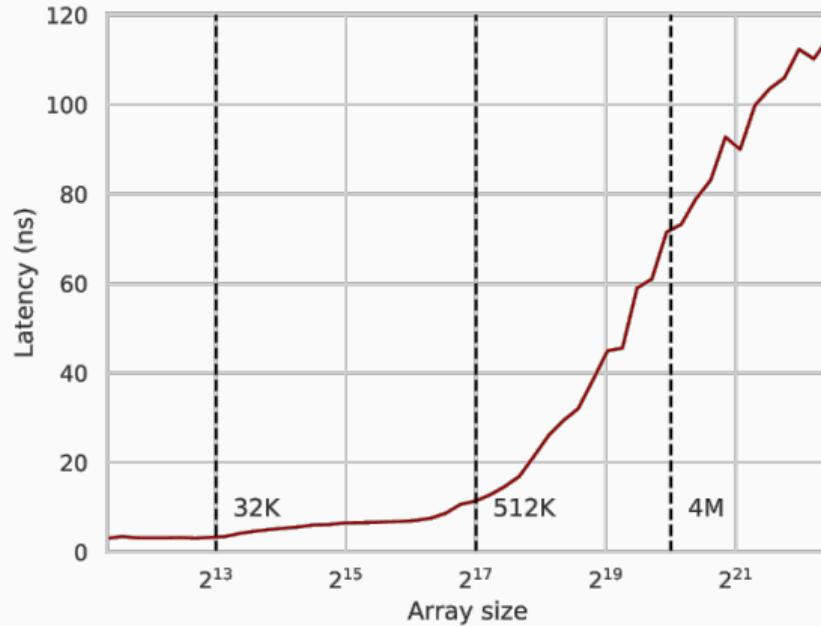
A **cache** is a small and fast memory located close to the processor that stores frequently used instructions and data. It is part of the processor package and takes 40 to 60 percent of the chip area
