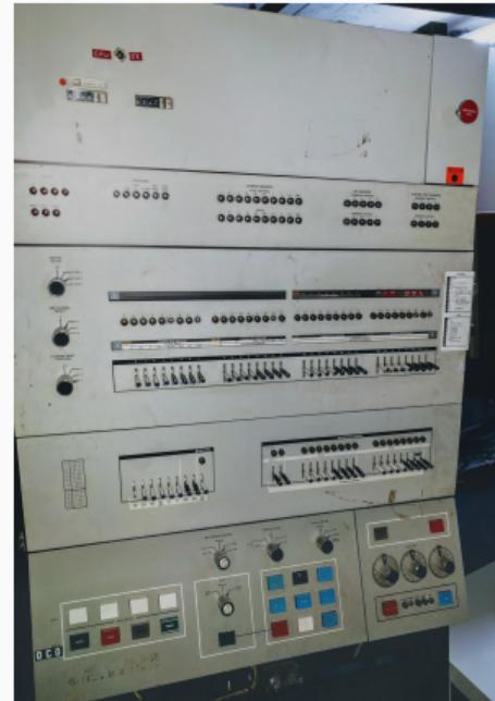
Ken Shirriff: Want to adjust your computer's floating point precision by turning a knob? You could do that on the System/360 Model 44
