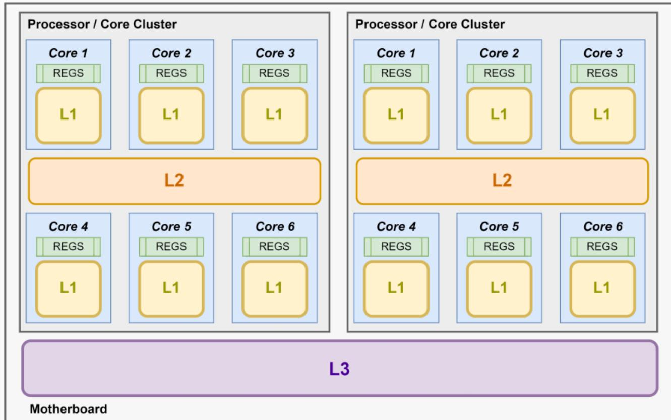
A **cache line** or **cache block** is the unit of data transfer between the cache and main memory, namely the memory is loaded at the *granularity* of a cache line. A cache line can be further organized in banks or sectors
